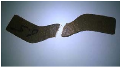
Fig.12. Composite specimen after Tear test.
