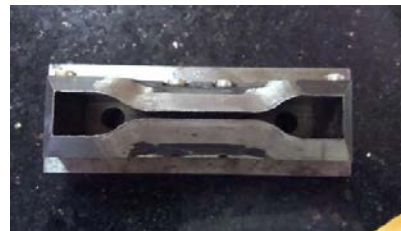
Fig.9. Die for Tensile specimen cutting.(ASTM).
